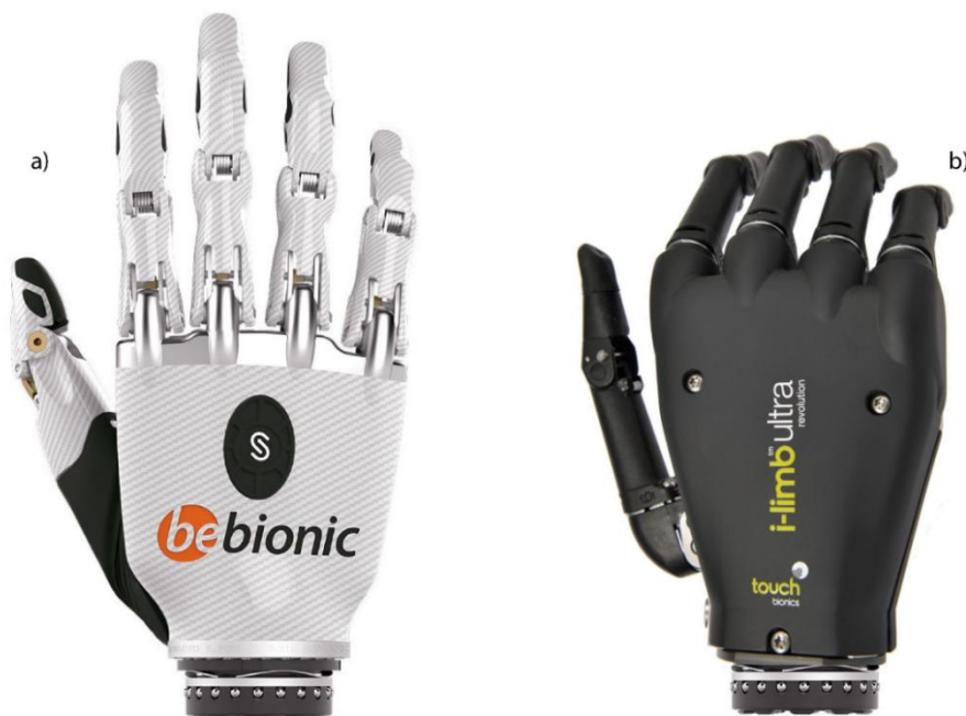
Figure 7. a) Bebionic3S prosthetic hand by RLS Steeper. b) Ultra-Limb prosthetic hand by Touch Bionics
