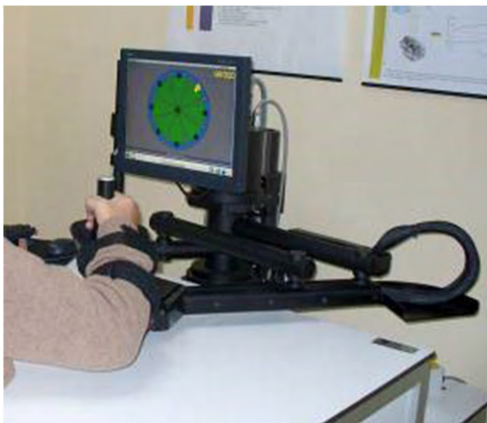
FIGURE 6.2: The InMotion2 robotic machine (Interactive MotionTechnologies, Inc.) employed in the study
