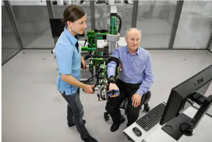
FIGURE 5.8: Rehabilitation session with the ARMin robot
