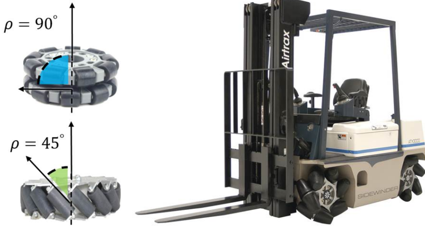
Figure 5.1: The figure reports the two typical mechanical layouts that are featured by an omnidirectional wheel (a): Omniwheel type is displayed on the top and Mecanum or Swedish wheel is displayed on the bottom. On the right (b), an example of a commercial vehicle equipped with omnidirectional wheels.
