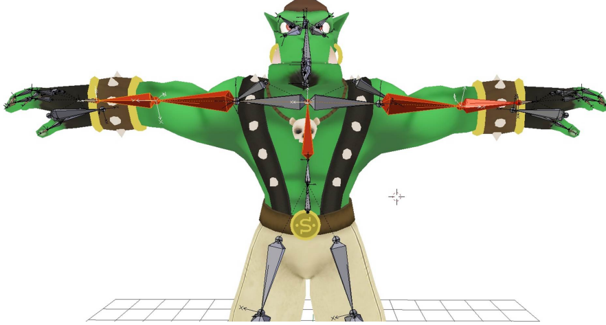
Figure 6.10: The figure shows the kinematic chain implemented for the avatar used for motion reconstruction of the upper body kinematics. All joints are set as ball in a socket type. Orientation data from the wearable IMUs are mapped to the movable segments (in red) through the estimated calibration matrix.
