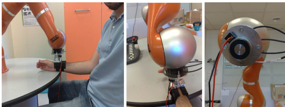
FIGURE 5.2: The designed mounting flange for connecting the robot end-effector and the patient's wrist
