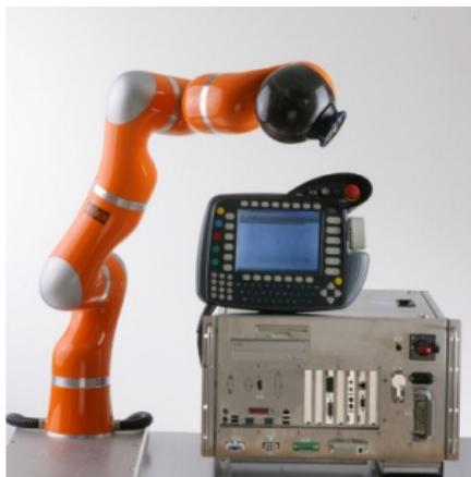
FIGURE 5.1: KUKA Light Weight Robot with robot controller (KRC 2lr) and control panel (KCP)
