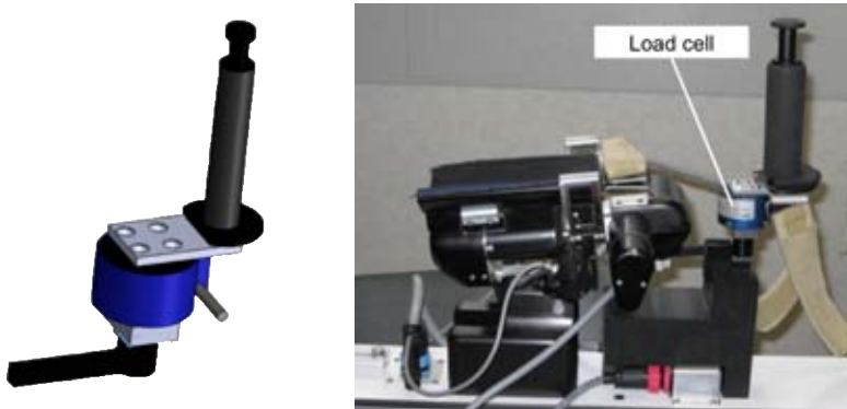
Figure 2.2: Integration of the force/torque sensor in the InMotion 3 system.
