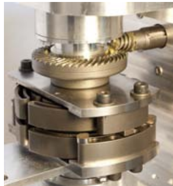
Figure 4.25: Picture of the assembled SEA prototype: the frame is fixed to an aluminum block, while the actuator output shaft is connected to a thin rectangular link..
