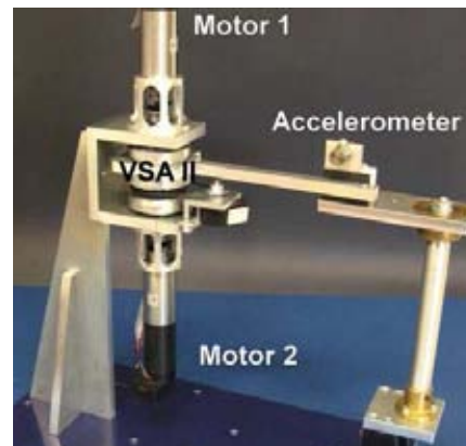
Figure 3.19: VSA-II prototype and experimental set-up [82].
