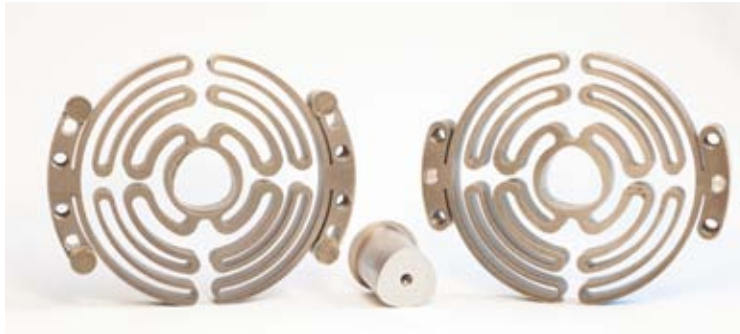
Figure 4.23: Picture of the custom torsion springs composing the spring pack. Dimensions: 80 mm external diameter 10 mm axial length. A shaped shaft-hub coupling based on P3G polygon is used as connection between the two springs internal rings. Steel mechanical hard stops are visible.
