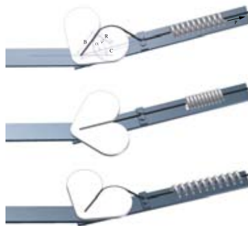
Figure 3.20: Working principle of the MACCEPA 2.0 [88].
