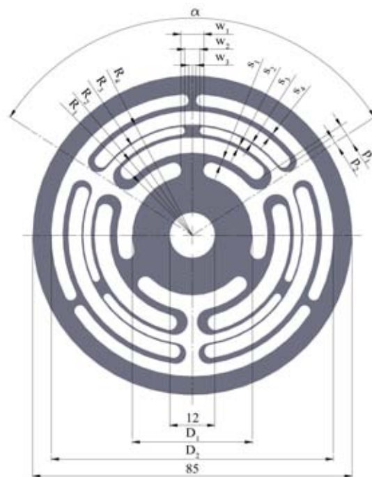
Figure 4.6: Drawing of a general spring morphology based on the selected topology with fixed and variable parameters. Letter are used for open parameters while number indicate fixed dimensions in mm. Disc thickness is a design constraint and is set to 3 mm. Radii of arches joining two different lamellae are not reported since are not independent variables.
