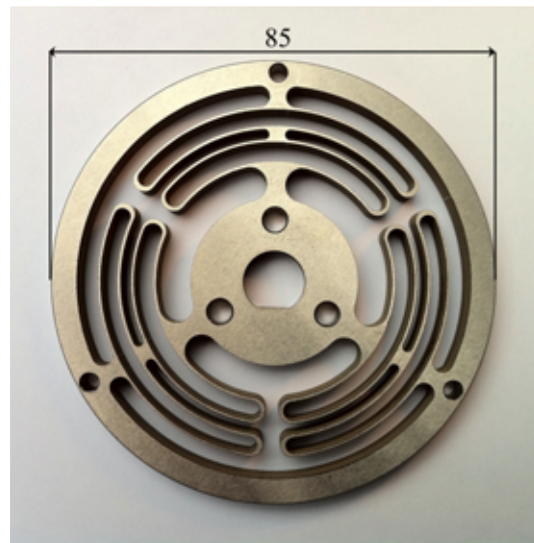
Figure 4.7: Picture of the custom torsional spring. Dimensions: 85 mm external diameter, 12 mm internal ring diameter and 6 mm axial length. A shaped shaft-hub coupling is used as connection between the spring internal ring and the output shaft.
