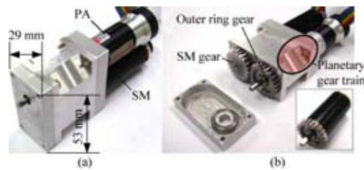
Figure 3.8: Prototype of the SDAU (a) and internal view of the planetary gear train (b) [63].
