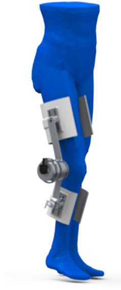
Figure 6.3: CAD drawing of an assistive knee orthosis integrating the presented SEA.
