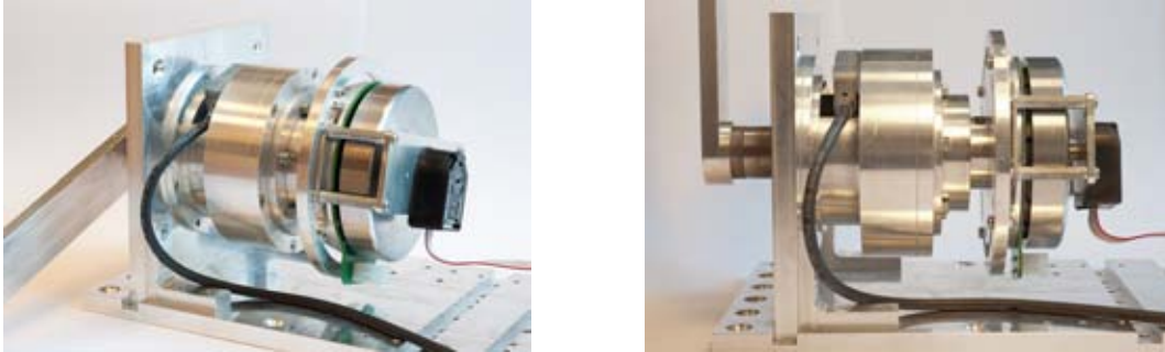
Figure 4.4: Picture of the assembled SEA prototype: the frame is fixed to an aluminum support, while the actuator output shaft is connected to a rectangular link.
