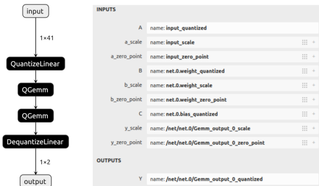
FIGURE 3.14: The ONNX graph of the Quantized MLP model. The QGemm, as a Q-Unit, presents attributes specific to linear quantization, consequently used by the compiler for generating C code.
