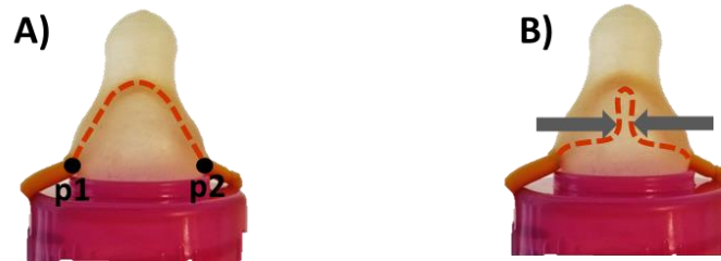
Fig. 25 A) The compressible rubber catheter is placed inside the teat forming a U-shape; the tube enters the teat through two diametrically opposite points ( p1 and p2 ), that are required to be placed in the middle of the infant's lips while measuring. B) Full catheter compression is achieved when the teat is totally compressed.
