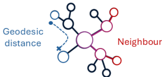
Figure 2.3: Nodes proximity is evaluated at a edge-level by using statistics that are based on the geodesic distance between two nodes (in blue), that is the length of the shortest path connecting them, or by assessing the similarity according to their neighboring nodes (the two red nodes interstate in their 2-hop neighbours in the purple node).
