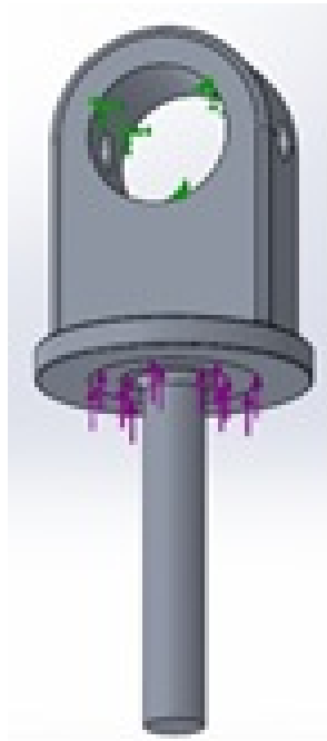
Figure 4.58: Loads and constraints imposed to execute the static analysis to obtain the best value for thickness of the male and female of the piston.
