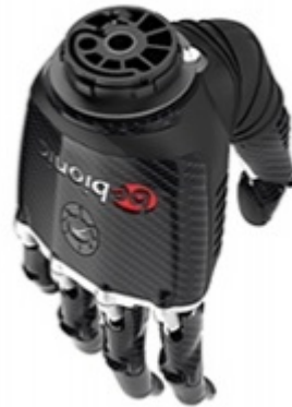
Figure 2.10: “Short” module for Bebionic 3 hand.
