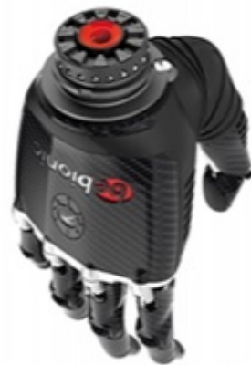
Figure 2.15: Quick release module for Bebionic 3 hand.
