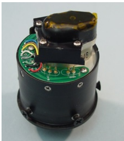
Figure 2.30: Active rotational wrist of LTI.
