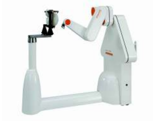
Figure 12: The NeuroMate™ robot system (Integrated Surgical Systems, Davis, CA).
