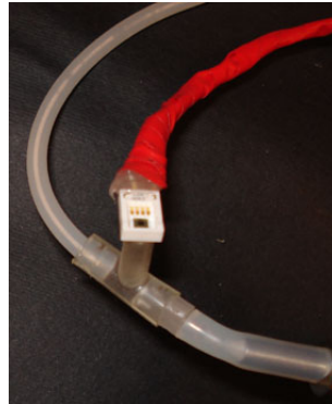
Figure 3.30: Detail of the MPX2300 pressure sensor mounted upstream of the damper.
