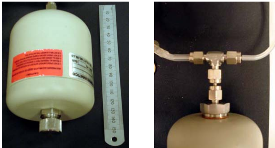
Figure 3.29: Left: the outside part of the elastic damper fabricated by Saip srl ( www.saip.it/ ). Right: detail of the Parker fluid connector used for connecting the damper with the rest of the hydraulic circuit.
