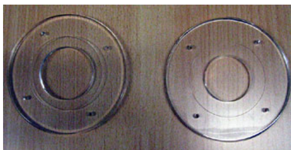
Figure 3.25: Two plexiglass modules that have been fabricated in order to vary membrane dimensions and, therefore, system compliance
