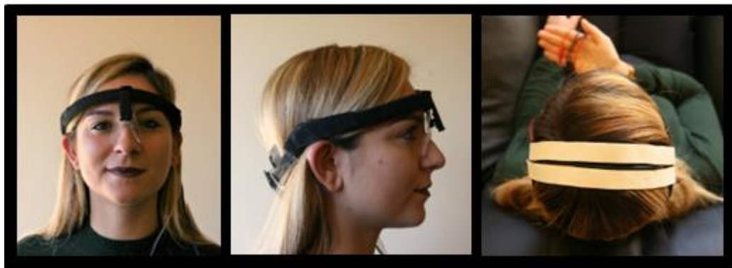
Fig. 2 The adaptable helmet consists of a simple customizable perimeter that can be applied with extreme precision to the tops of the ears and the base of the nose. The occipital cathode is placed in the posterior while Velcro bands are employed to hold the anode electrode on the S1 area. (Figure and caption reformulated from Tecchio et al. 2022).
