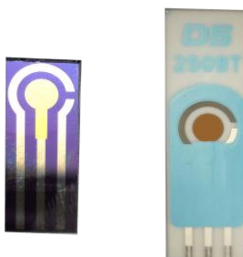
Figure 23: Micro-fabricated electrode (left) and Commercial screen printed electrode (right)
