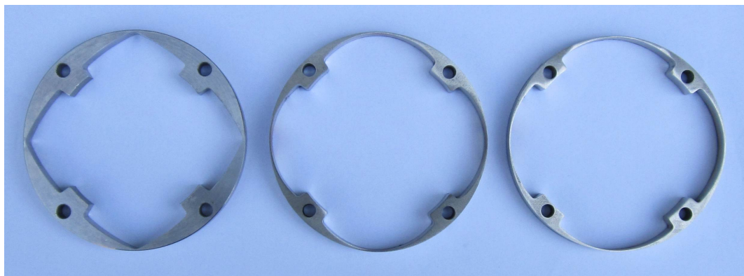
Figure 3.41: Cam discs with constant, linear and quadratic stiffness-angle characteristics (from left to right).
