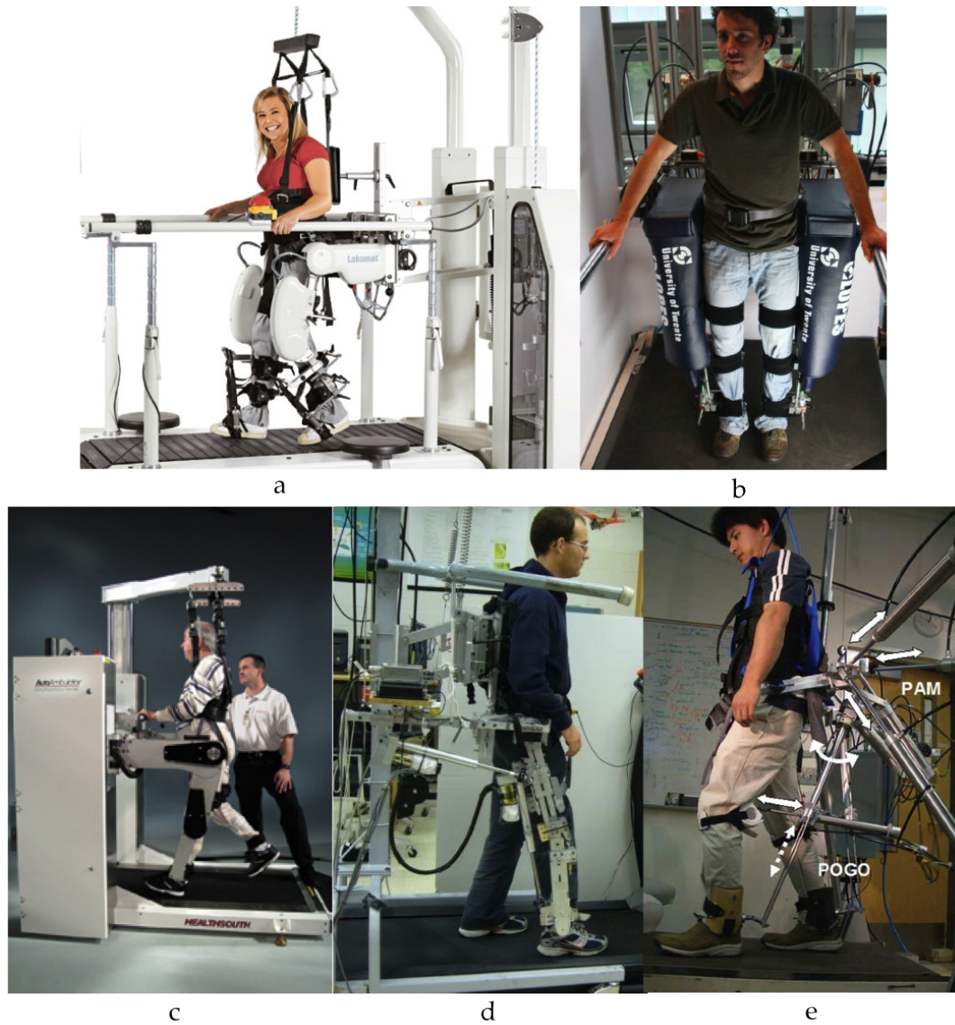
Figure 2.6: Treadmill-based exoskeletons for rehabilitative purposes. (a) Lokomat, (b) LOPES, (c) AutoAmbulator, (d) ALEX, (e) PAM-POGO.
