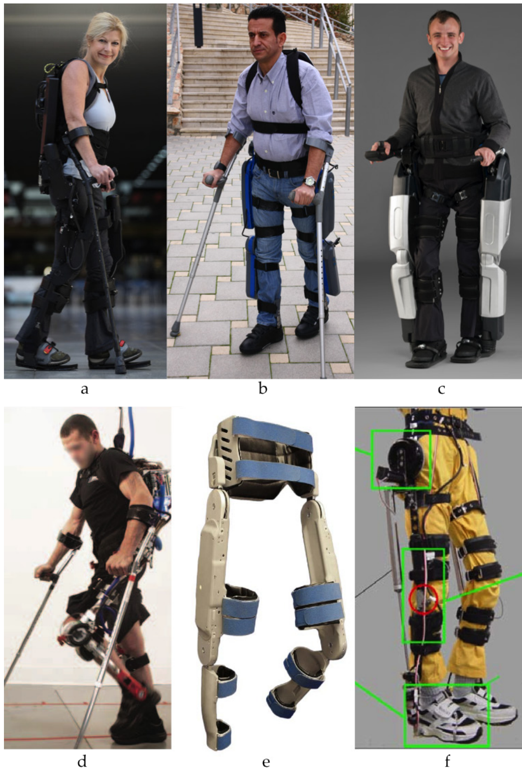
Figure 2.5: Mobile medical exoskeletons for rehabilitative and assistive purposes. (a) Ekso, (b) ReWalk, (c) REX, (d) MINA, (e) Vanderbilt powered orthosis, (f) Wearable Walking Helper.
