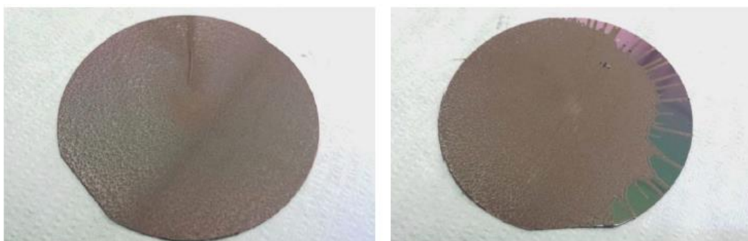
Figure 29 C-PDMS at 2000 and 2500 rpm
