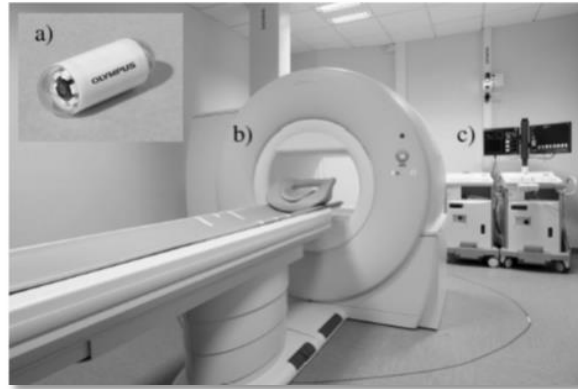
Figure 8 Magnetically Guided Capsule Endoscope with a) capsule endoscope b) magnet guidance c) user interface [61].
