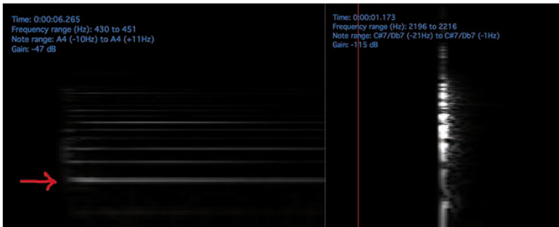
Figure B.9. Frequency analysis of a musical tone (A4 from a piano, left) and a noise (wooden hammer banging on a table, right). Vertical axis = frequency. Horizontal axis = time. A fundamental frequency (arrow) and harmonics at higher frequencies can be recognised on the left. Image generated with WavePad software.
