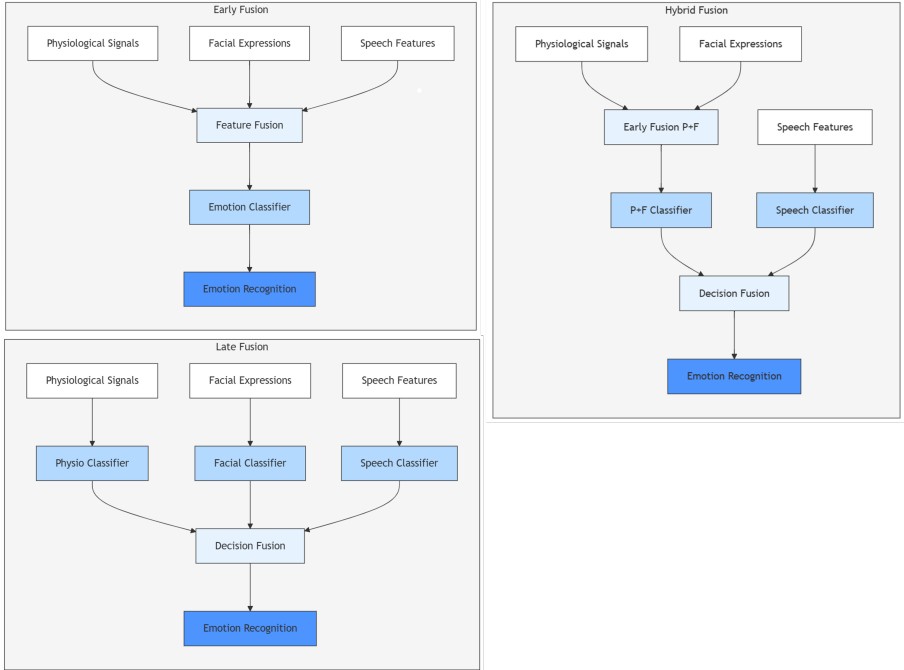
Figure 3.11. Comparison of multimodal fusion architectures for emotion recognition. Early Fusion (top left) combines physiological signals, facial expressions, and speech features at feature level; Late Fusion (bottom) processes each modality through dedicated classifiers before decision-level fusion; and Hybrid Fusion (right) merges physiological and facial data early while processing speech separately. Color intensity indicates processing stage: input features (white), intermediate processing (light blue), and emotion recognition output (dark blue).
