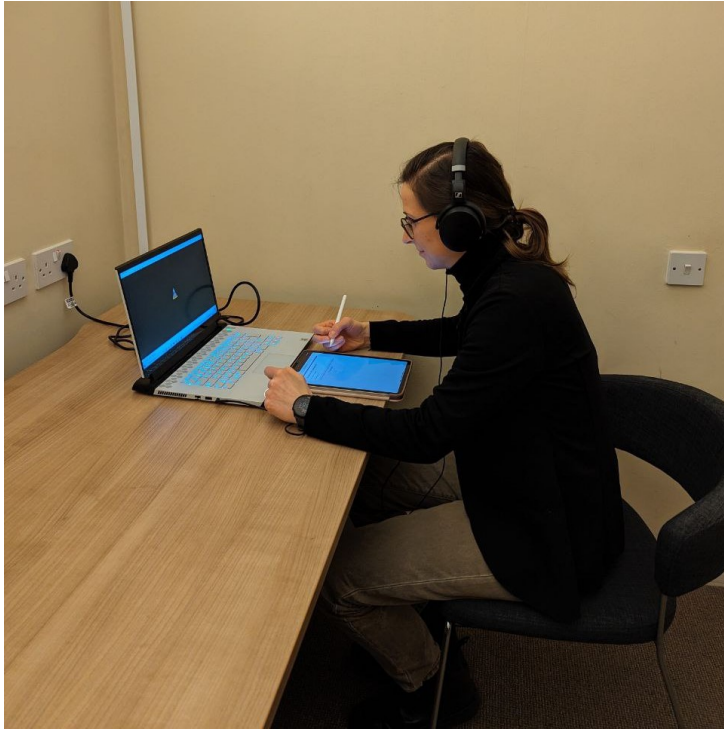
Figure 3.18. Experimental setup showing participant using the tablet for SAM scale ratings while wearing Empatica E4 wristband for physiological measurements and Sennheiser HD 450BT headphones for audio playback. The laptop screen displays video stimuli while the integrated webcam records facial expressions.
