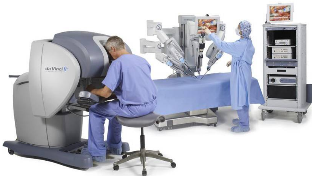
FIGURE 3.6: The Da Vinci telesurgical master-slave robot [128].
