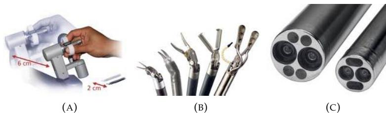
FIGURE 3.7: a) The motions of the slave arms are controlled by the surgeon through controllers; b) Interchangeable EndoWrist can be mounted on the slave arms end-effectors; c) Endoscopic optics provide the surgeon with a 3D view of the operating site. Acting on a foot pedal the surgeon can zoom in and zoom out the scene [128].
