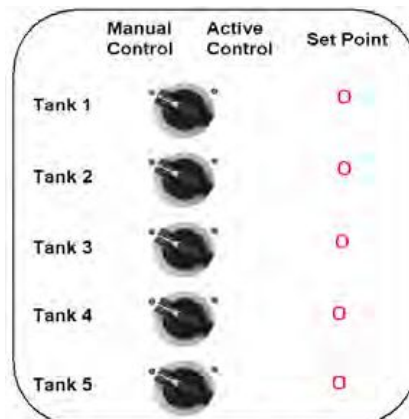
FIGURE 6.33: Automatic level control panel
