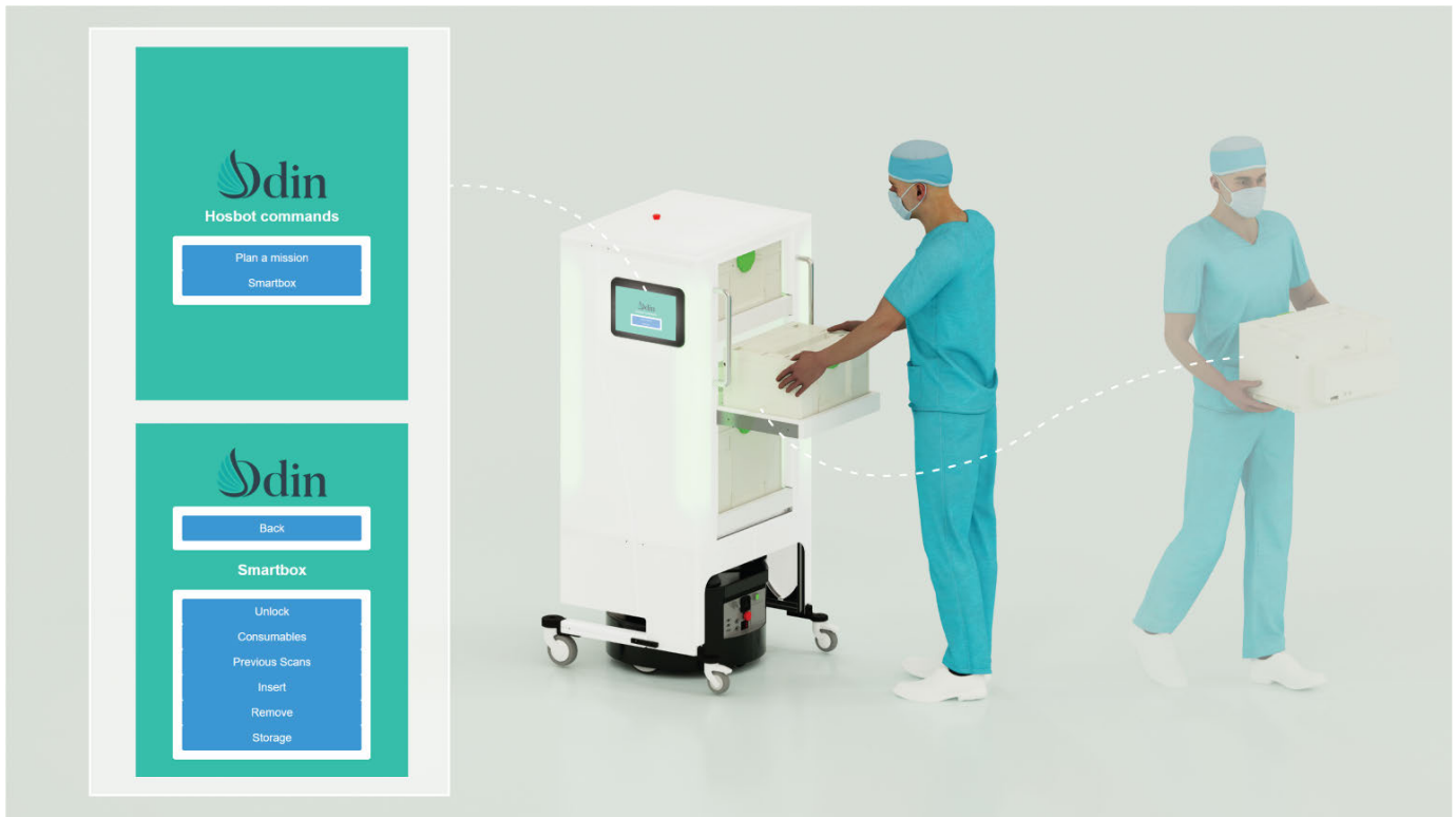
Fig. 6. The HOSBOT HMI is available on authorised edge devices and on the SmartRack tablet. The starting page allows users to plan a HOSBOT mission or interface with the SmartBoxes. Once the SmartBox button is pressed, a menu is shown, allowing to unlock specific SmartBoxes, monitor consumables within them, perform a scanning operation of the included content, consult previous scans, and insert/remove objects. SmartBoxes are standalone devices and can be withdrawn from the SmartRack upon user authorisation.
