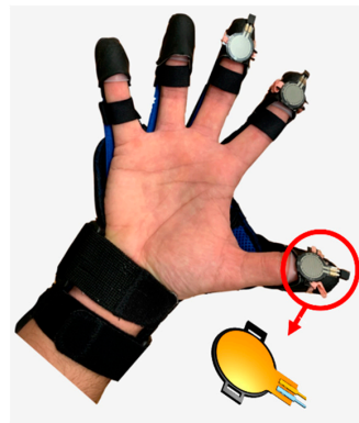
Figure 2. Force sensors positioned at the fingertips of Gloreha Sensor Glove.
