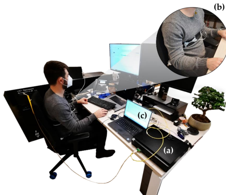
Figure 4.9. Representation of the experimental setup: (a) the FBG interrogator, (b) the elastic band instrumented with two flexible sensors and (c) the laptop dedicated to the acquisition of data from the interrogator.
