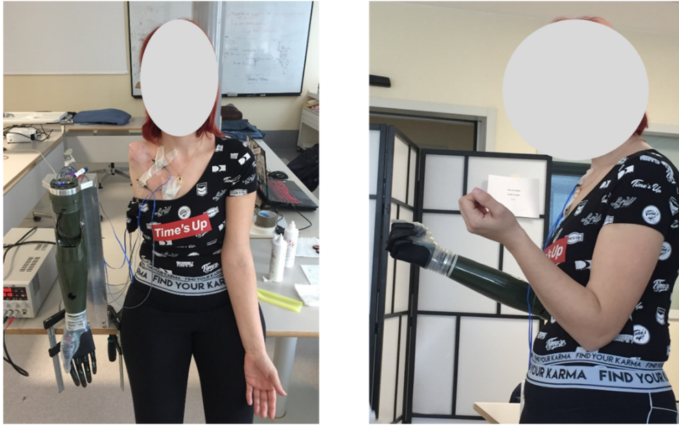
Figure 4.11: The TMR patient control the bench prosthetic system composed of three different modules: the elbow with active flexion/extension (Hosmer); the HANNES hand; the wrist with active pronation/supination (Ottobock).
