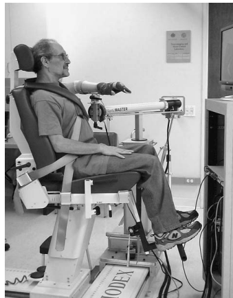
Fig. 5: ACT-3D rehabilitative robot
